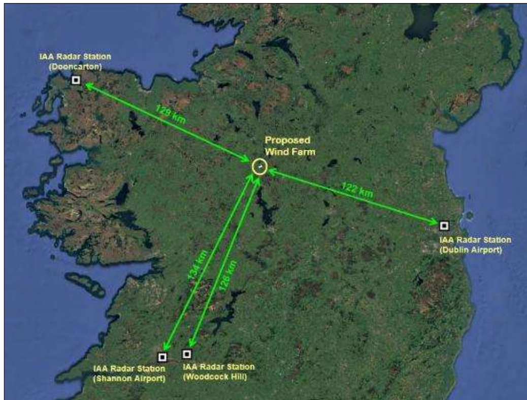
Figure 8. Radar Surveillance Sites relative to Ballyfeeny wind farm site.
